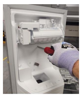
**Step 4:** Pull the bottom of the icemaker assembly toward you and the whole assembly will move forward and drop down exposing the wiring harness at the top:
