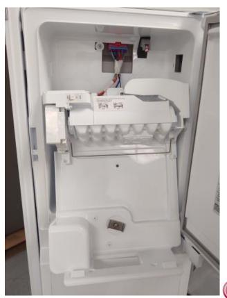
**Step 5:** Press down on the release tab located on top of the wiring connector and unplug the connector from the door:
