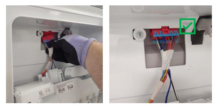
**Step 2:** Push the icemaker assembly back into place. Notice that there is an alignment tab at the top. The U-Shaped cutout in the top of the icemaker will slide behind the tab. To install, push the icemaker up and back into place:
