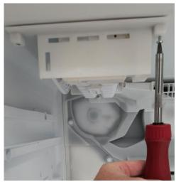
**Step 4:** After removing both screws pull the icemaker straight down from the front and once the front is loose pull the icemaker forward to uninstall from the rear mounts:
