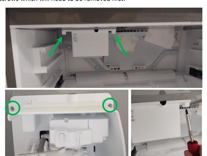
**Step 4:** After removing both screws pull the icemaker straight down from the front and once the front is loose pull the icemaker forward to uninstall from the rear mounts:
