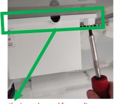
\*\*Note: Make sure once Icemaker is reinstalled that there are no gaps between the icemaker and freezer liner.
