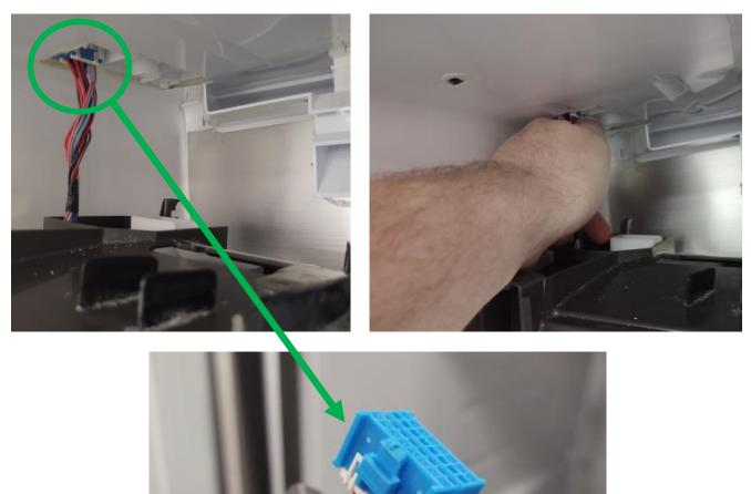
**\*\*Note:** The release tab is located on the left side of the connector and in some cases there is not much room to get your finger on the tab to press it. In that case use a short flat blade screwdriver to press in on the tab so it will release from the connector:
