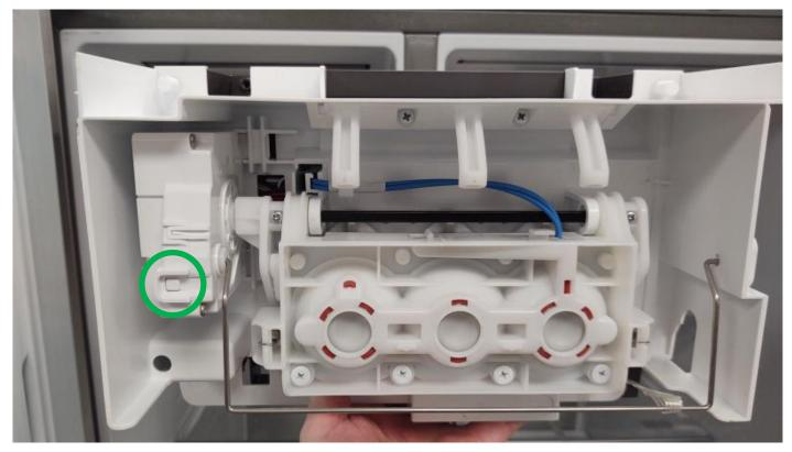
**Step 6:** Snap the decorative cover back into place, all 4 corners should be secure if installed correctly, Simply press the cover toward the icemaker and you will hear it snap into place:
