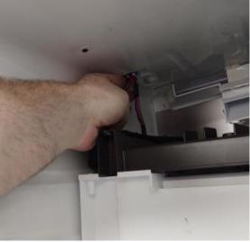
**Step 2:** Position the icemaker back into place. There is a hanger located on the top left side of the icemaker and another on the right side of the icemaker. Make sure the back of the icemaker is resting on these hangers:
