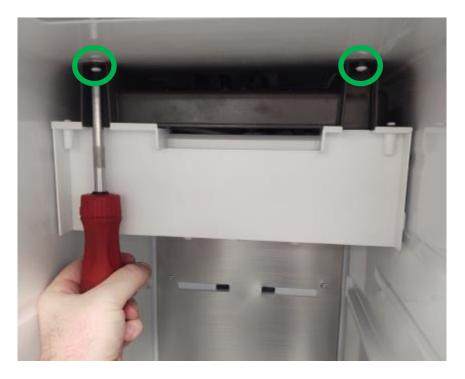
**Step 4:** After removing the 2 screws pull the icemaker toward you and down and the right side will rest on the upper shelf holder:
