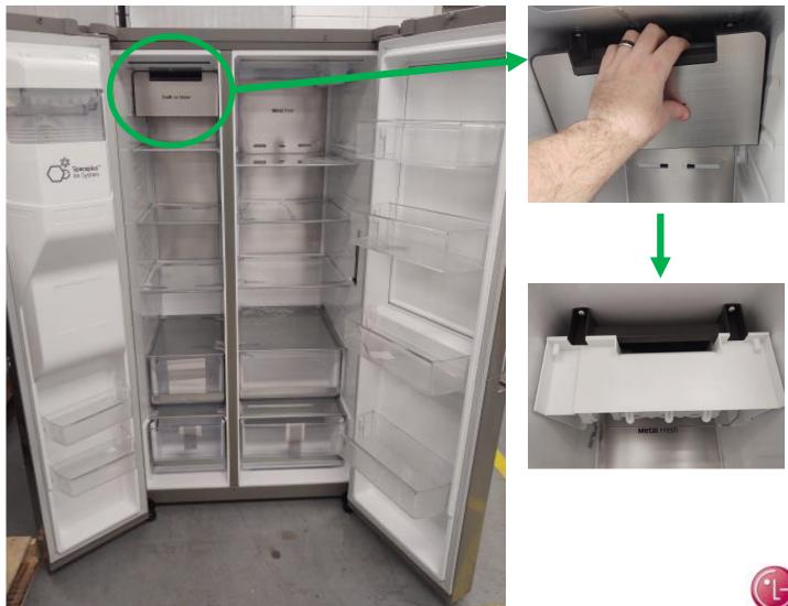
**Step 3:** Remove the 2 phillip screws that are securing the icemaker to the ceiling of the unit:
