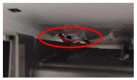
**Step 4:** With Icemaker in position and wires safely tucked away you can reinstall the 2 Phillips screws that secure the front of the icemaker to the liner:
